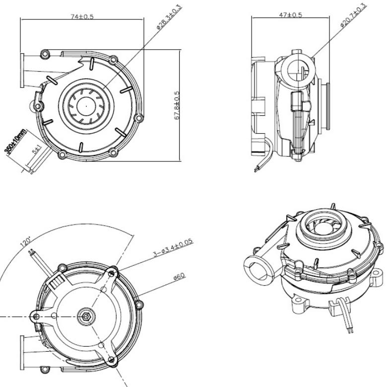
LEAD WIRE UL 1007 20AWG OR EQUIVALENT
